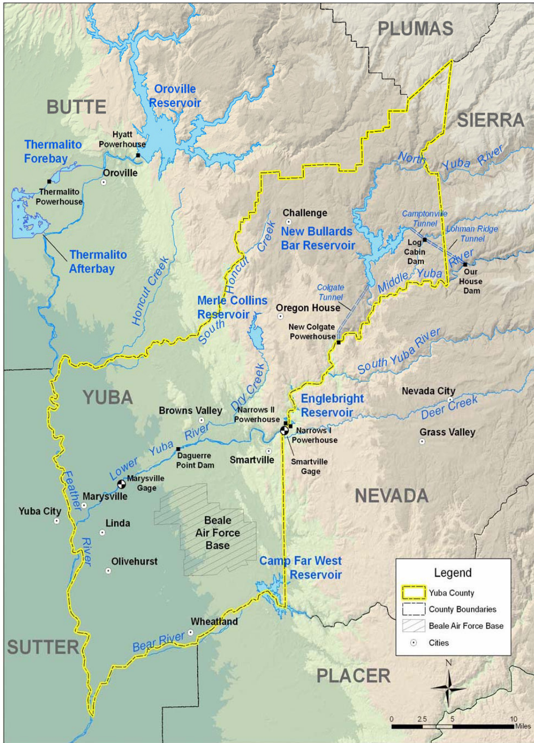
Figure 1-1. Major Water Development Facilities in the Lower Yuba River Basin
